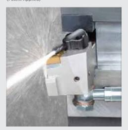
**SmartFlow** ensures that the Block where tool is performing machining operation gets 100% of pump flow & pressure.
