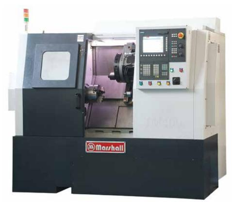
60 Degree True slant bed Structure with "Torque Tube" for additional rigidity
