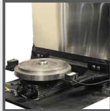
Gauging Station with Twin Laser for diameter & ovality measurement
