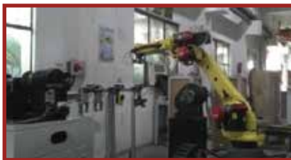
Robot drops Shaft Gripper set on its stand & goes to pick gear blank gripper set
