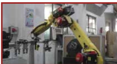
Robot wrist attaching to vision sensor.
