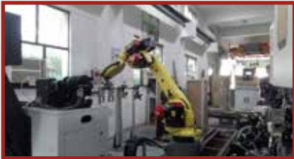
Robot wrist attached to one set of 'Quick change' gripper for shaft handling.
