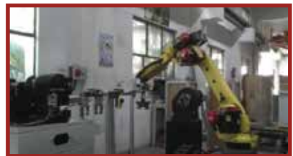
Robot wrist attached to new set of 'Quick change' grippers for Gear Blank handling.
